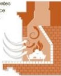
A conventional firebox allows a fraction of the radiant heat out because of its depth and angle of the walls.
