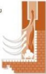
A Rumford firebox will maximize the radiant energy of the fire due to its shallow depth and optimally angled sides.
